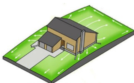
Ideal Water Runoff
